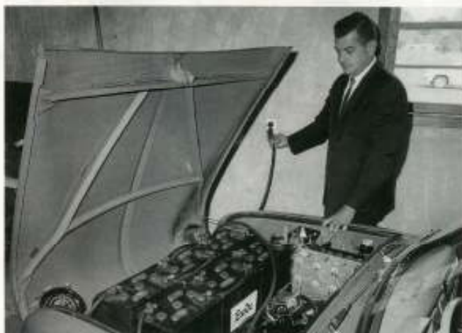
A single 25-foot cable serves all three chargers, and is conveniently stored under the hood.
