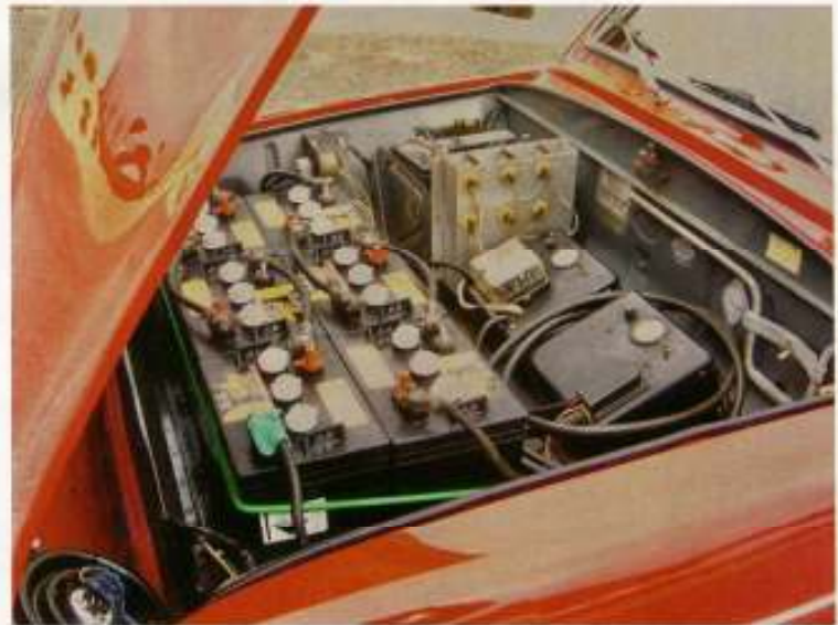
Front compartment of Henney with six 12-volt batteries. On the right, front to back, a 12-volt charger, a 72-volt charger, a heatsink, and a 12-volt control battery.
