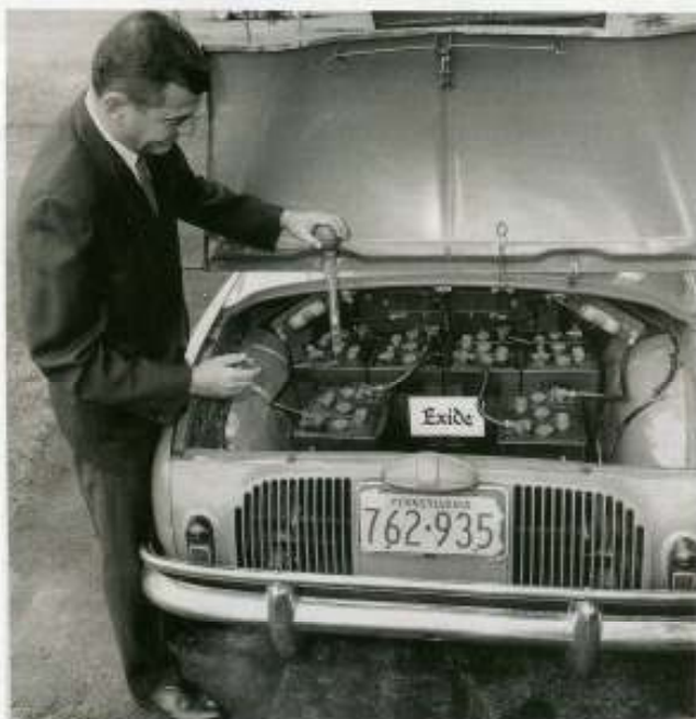
Performing a specific gravity check for troubleshooting.
