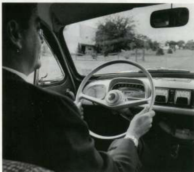
Simplified dash: Speedometer and odometer, two power indicators, and forward/neutral/reverse switch complete the uncomplicated Kilowatt dash.
